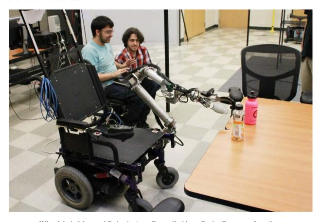
Wheelchair-Mounted Robotic Arm Controlled by a Brain-Computer Interface
